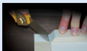
9. Cut a 45° angle slit on each corner.
